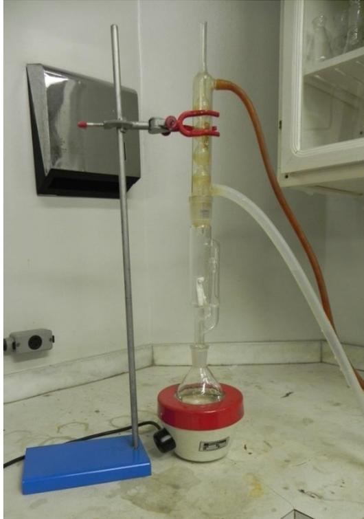
Figura 19: Extrator Soxhlet.
