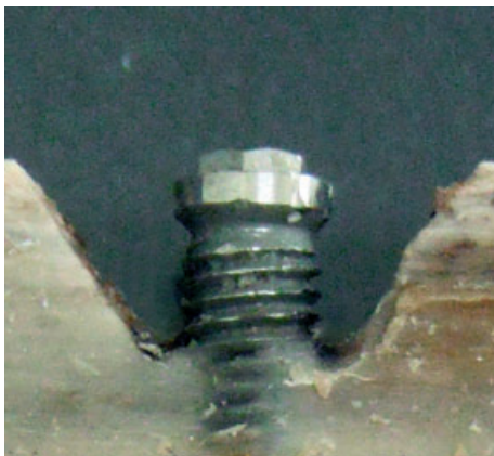
Fig. 1. The implants were placed into bovine ribs and the defects were created on both sides of the implants.
