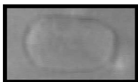
Fig. 2. Drop of MEG on rubbed PVA. It is oblong and stretched along the rubbing direction.
