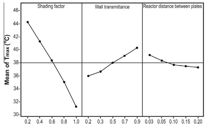
**Fig. 2.** Mean values for tested parameters and reactor maximum temperature.
