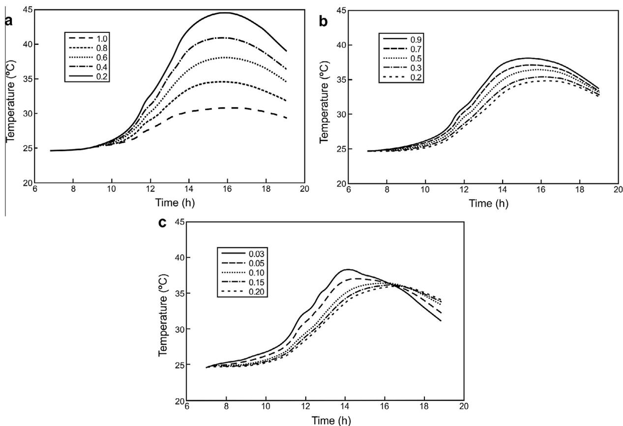
Fig. 3. Variation in the culture medium temperature for (a) shading factor range 0.2–1.0, (b) reactor wall transmittance range 0.2–0.9 and (c) reactor distance between plates ranges 0.03–0.2 m.
