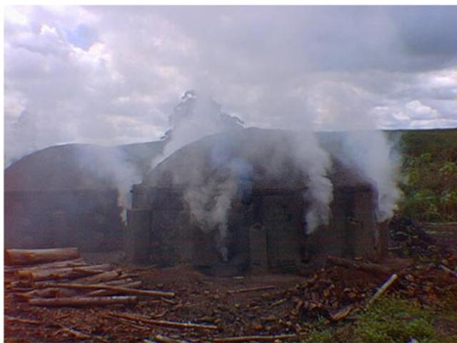
**Fig. 1** A single kiln during the combustion process
