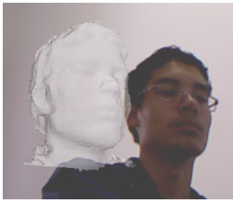
Fig. 6. An example of tracking failure. The user needs to reposition his face to the tracking algorithm align correctly the raw depth data to the reference 3D model.
