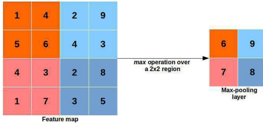
Figure 2.6: Example of a max-pooling layer obtained from an input or feature map.
