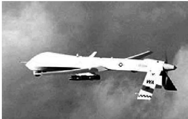
**Figura 1.1.** Predator com mísseis Hellfire, Airforce Technology (AIRFORCE..., 2006).
