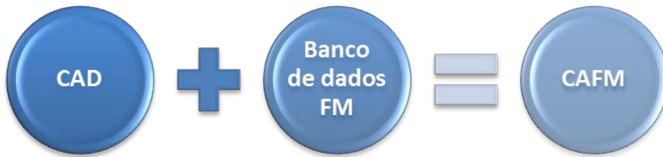
Figura 5 – Computer Aided Facility Management
