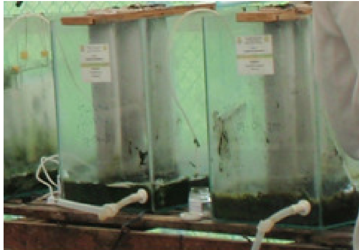
Figure 5: Aquariums with mixed microbial highlighting the dark color of the solution before forming the film.
