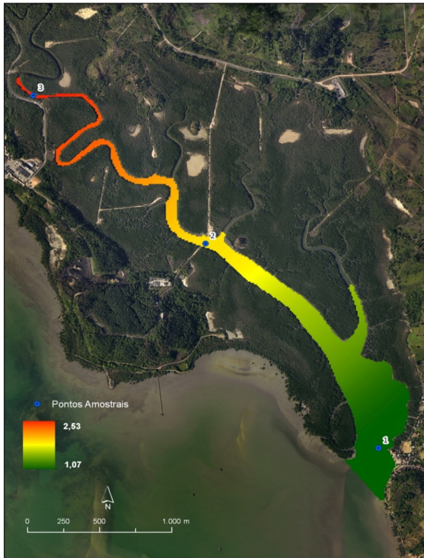
Fig. 14. Map of interpolation made by the Kernel method showing the variation in vulnerability to oil spills in São Paulo river.
