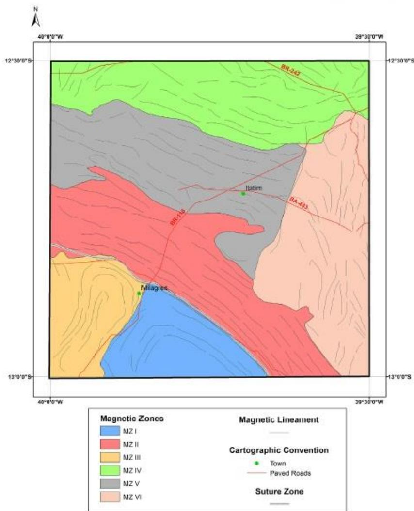
Fig. 11. Map showing the interpretation of magnetic zones and structural lineations derived from airborne geophysical magnetic data of the Milagres region.
