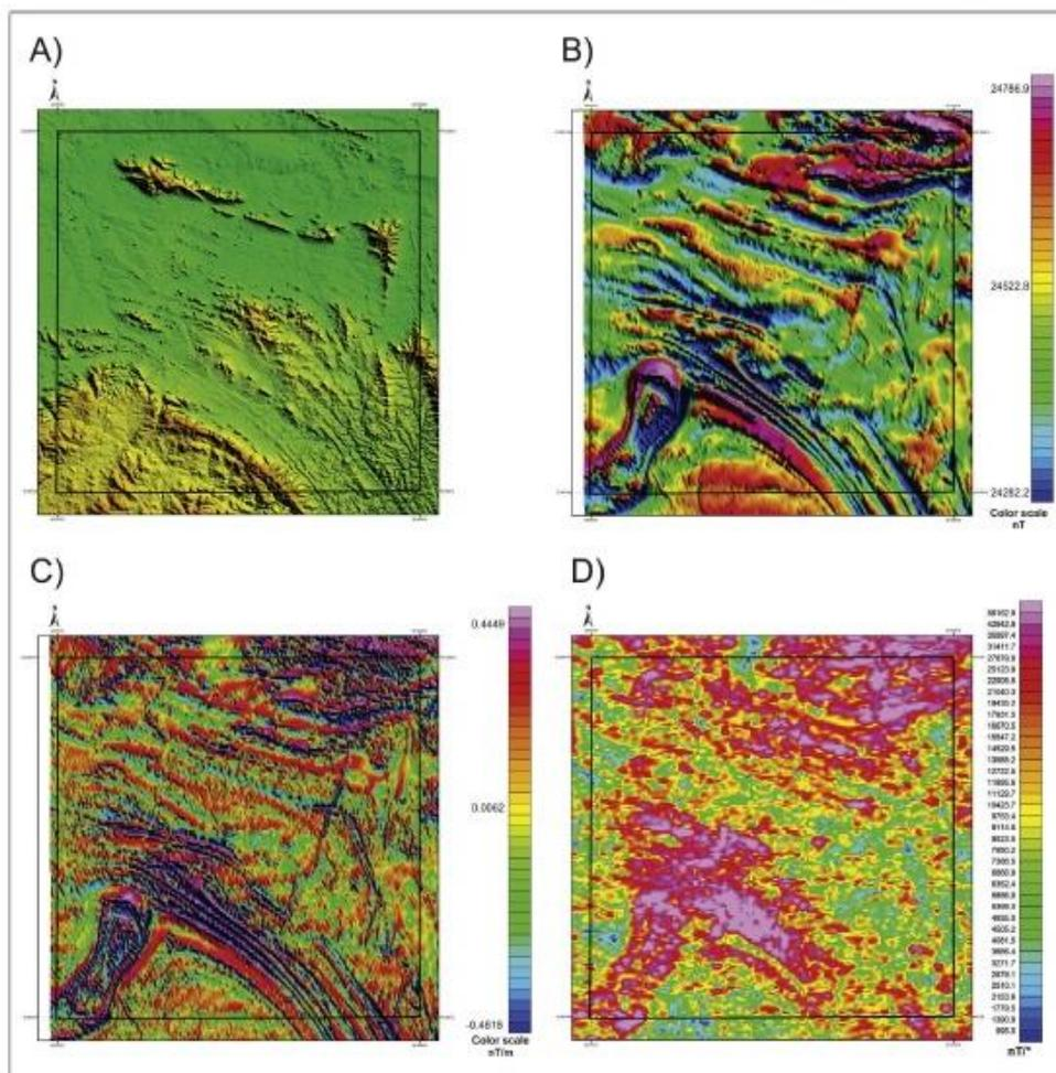
Fig. 10. (A) Digital terrain model map; (B) Total magnetic field intensity map; (C) Magnetic field first vertical derivative map; and (D) Analytical signal amplitude map.
