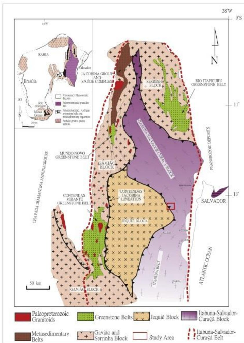
Fig. 3. Spatial arrangement of the main blocks that compose SFC. (A) Positioning in the state of Bahia; and (B) Representation of the limits between blocks, highlighting the present study area, at the limit between the Itabuna-Salvador-Curaçá Block and the Jequié Block.
