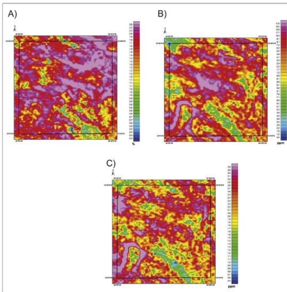
Fig. 7. Gamma-ray spectrometry airborne geophysical maps of the Milágres region. (A) K channel; (B) eTh channel; and (C) eU channel.
