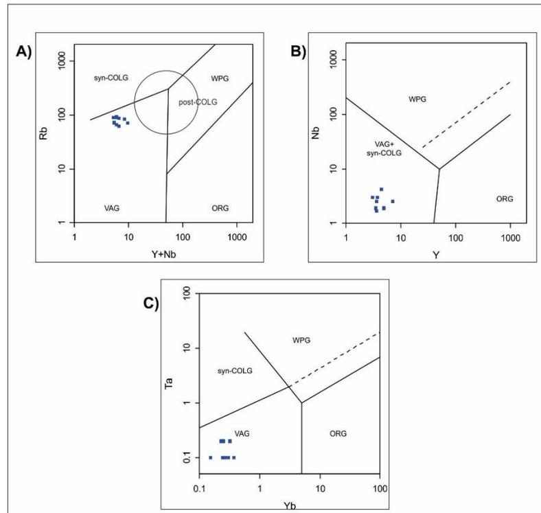
Figura 12 – Diagramas de classificação geotectônica de Pearce et al. (1984): A) diagrama Rb/Y+Nb; B) diagrama Nb/Y; e, C) diagrama Ta/Yb. (VAG: volcanic arc granites, COLG: collisional granites, ORG: orogenic granites, WPG: within plate granites).
