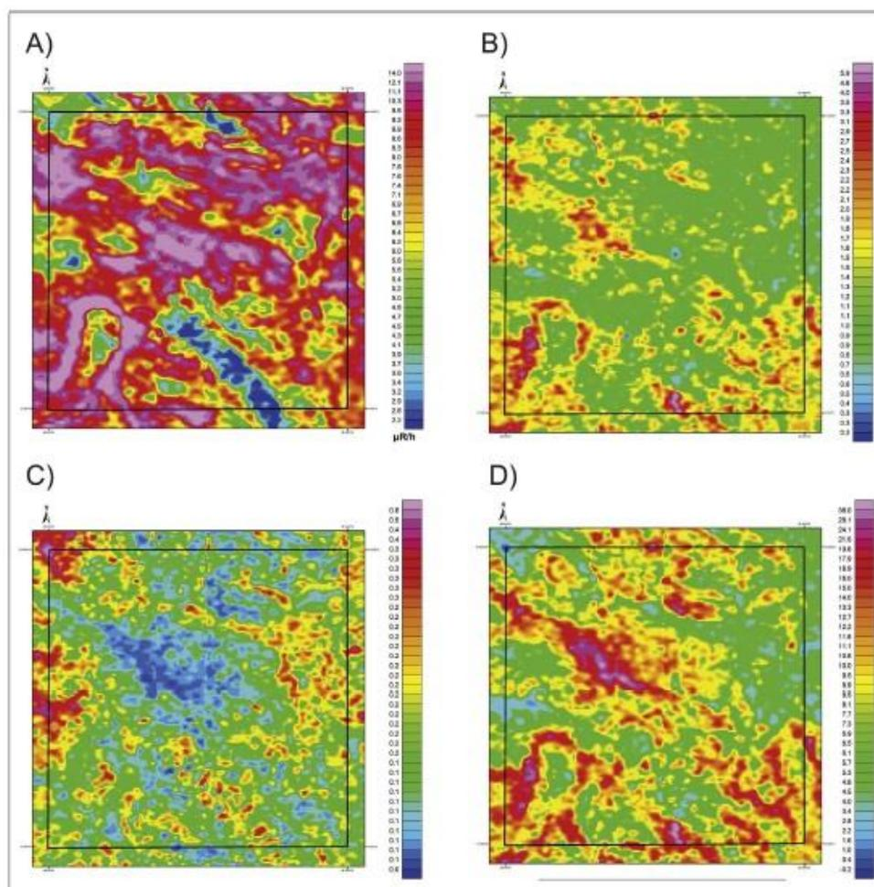
Fig. 8. Gamma-ray spectrometry airborne geophysical maps of the Milagres region. (A) Total count; (B) U/K ratio; (C) U/Th ratio; and (D) Th/K ratio.
