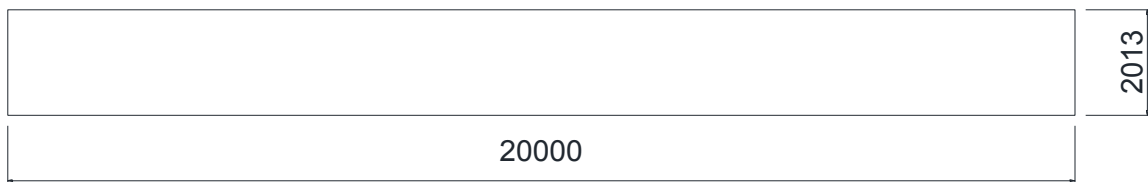
Figure 5: Side view and dimensions of the prismatic vessel – dimensions in “mm”
