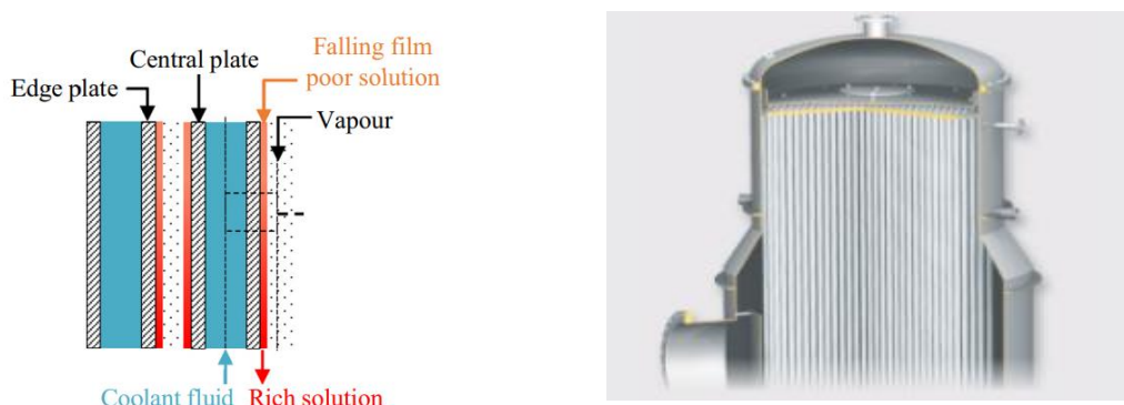
Figure 5- Falling film absorber: (a) plates (Triche et. al., 2017), (b) tubes (Gea, 2017).
