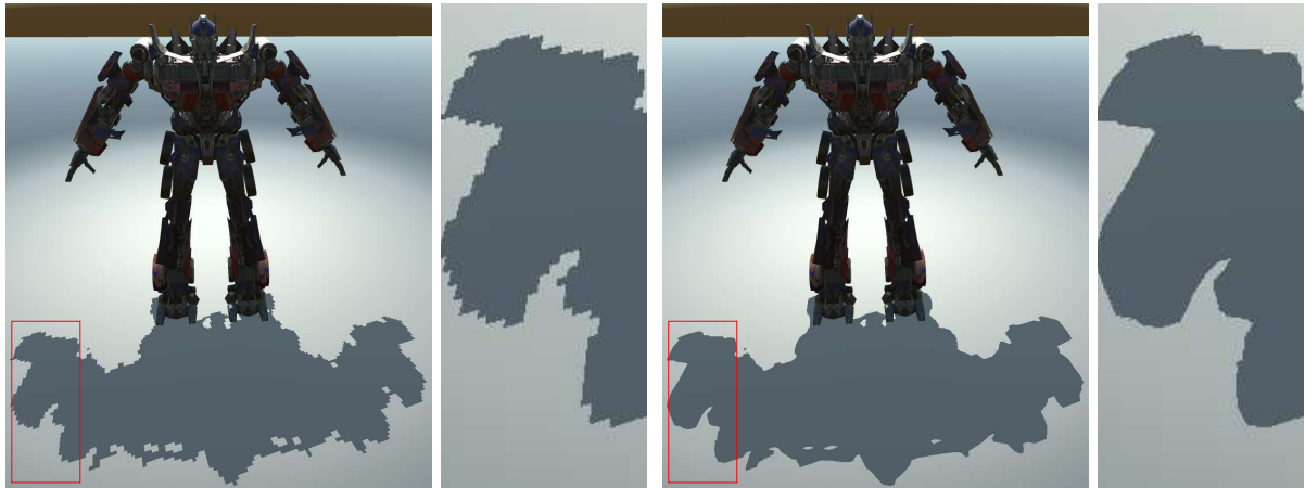
Figure 3.15 A visual comparison between shadow mapping (left) and conservative RBSM (right) for the Robot model using a 1024^2 shadow map resolution.
