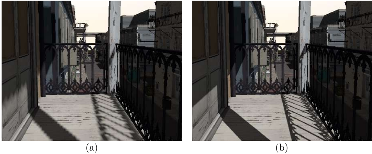
Figure 2.7 For a large scene, the use of an insufficient shadow map resolution may generate aliasing artifacts along the shadow silhouette (a). The efficient distribution of several high-resolution shadow maps per sub-units of the 3D space helps on reducing these aliasing artifacts (b). Images courtesy of (LAURITZEN; SALVI; LEFOHN, 2011).
