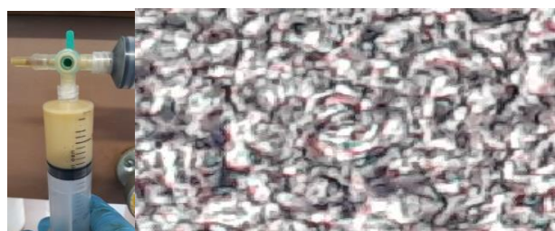
Figure 1: Detail of Lauer lock syringes connected / microcapsules contents of the geopropolis extract. Olympus optical model CX40RF100- Objetiva 100x.
