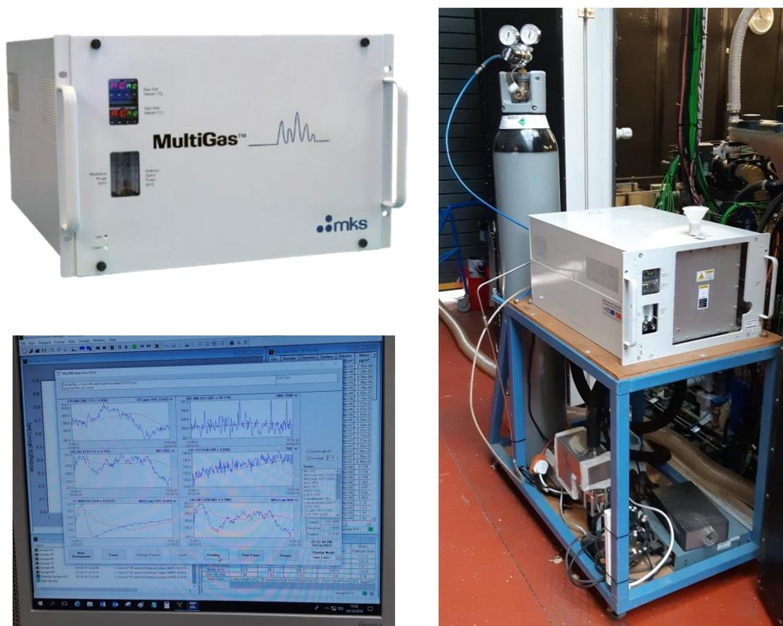
**Figure 19.** The FTIR equipment (top left), gas measurement screen (bottom left), and the assembling of the FTIR (right).
