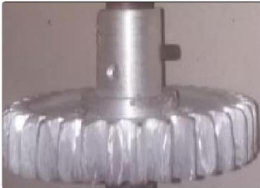
Figure 10. Gear 4 as cast.
