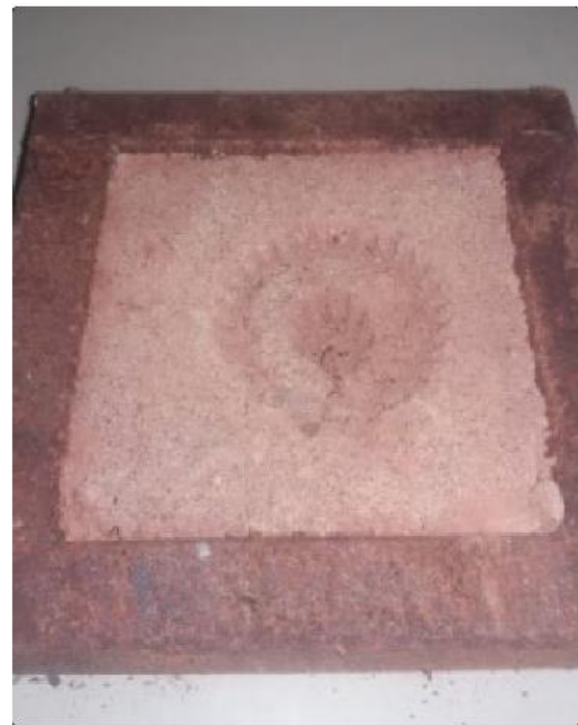
Figure 8. Sand mold for the first gear.
