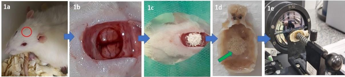
Figure 1. Experimental design. (1a) Place on the calvaria where the intervention was performed. (1b) Aspects of the critical bone defect model made with 8 mm in diameter. (1c) Exemplary of the glass-ceramic implant process. (1d) Calvaria specimen with implant in the central portion (green arrow), and (1e) positioning of sample in the FT-Raman system compartment.
