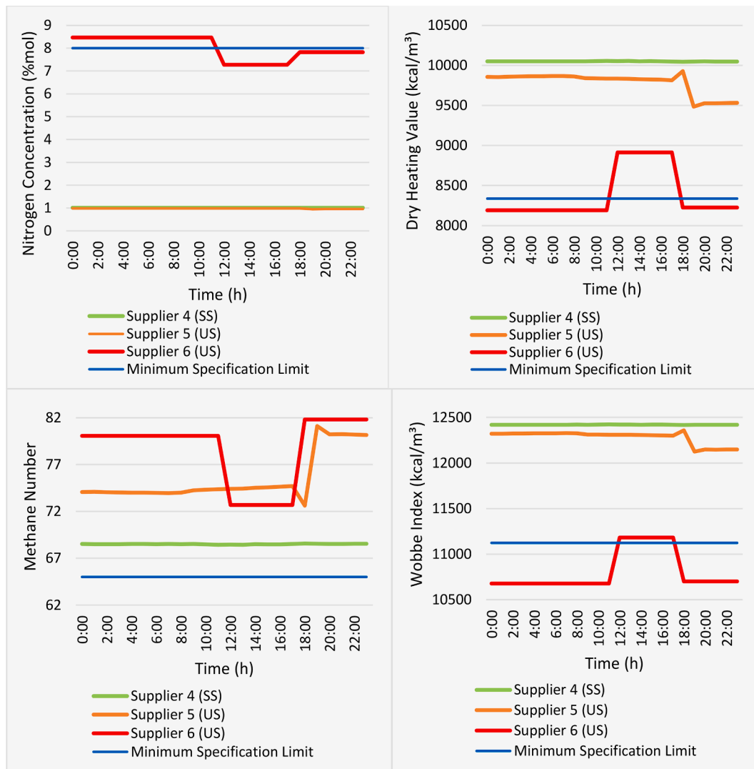
Fig. 13. Nitrogen concentration, heating value, Wobbe Index and methane number (mixture B).
