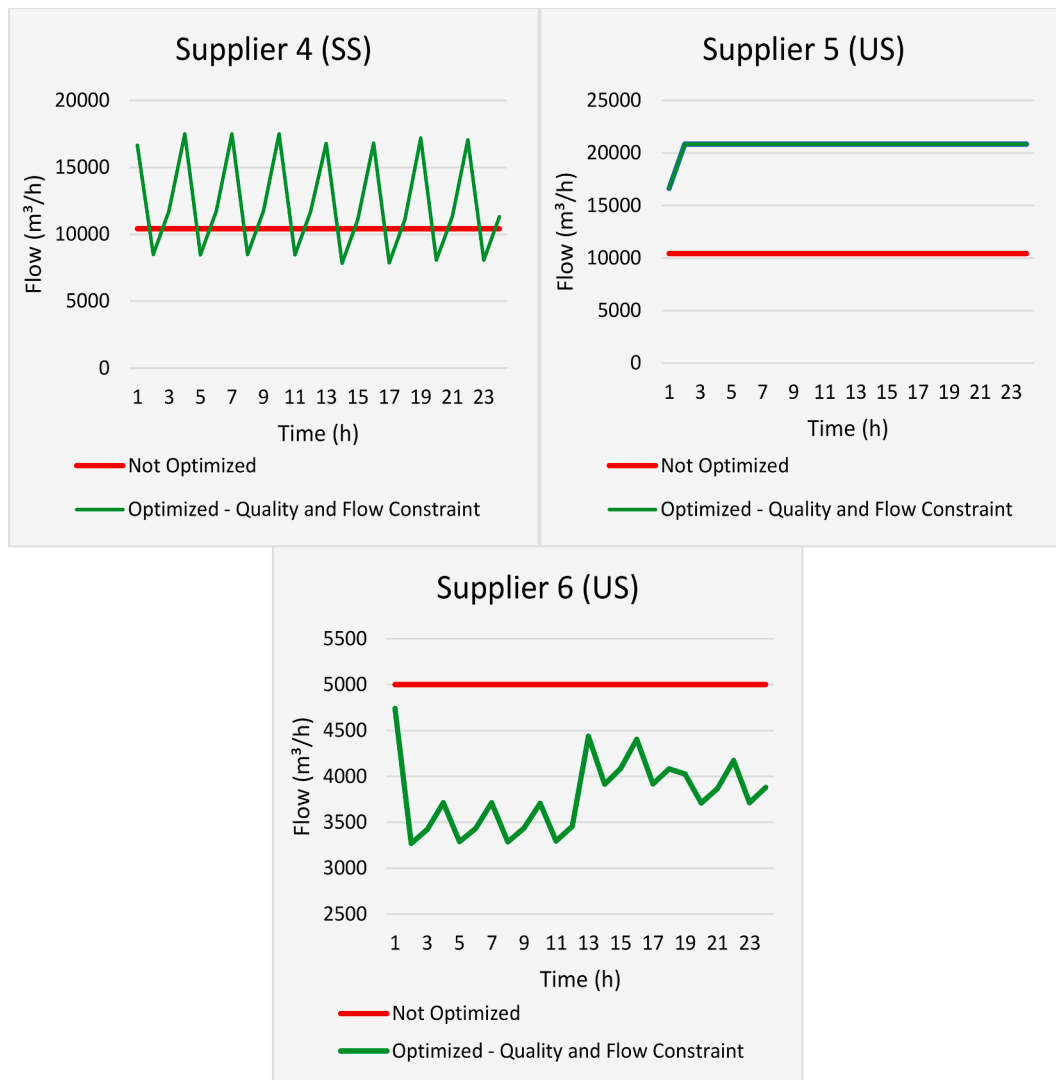
Fig. 14. Input flows (mixture B).
