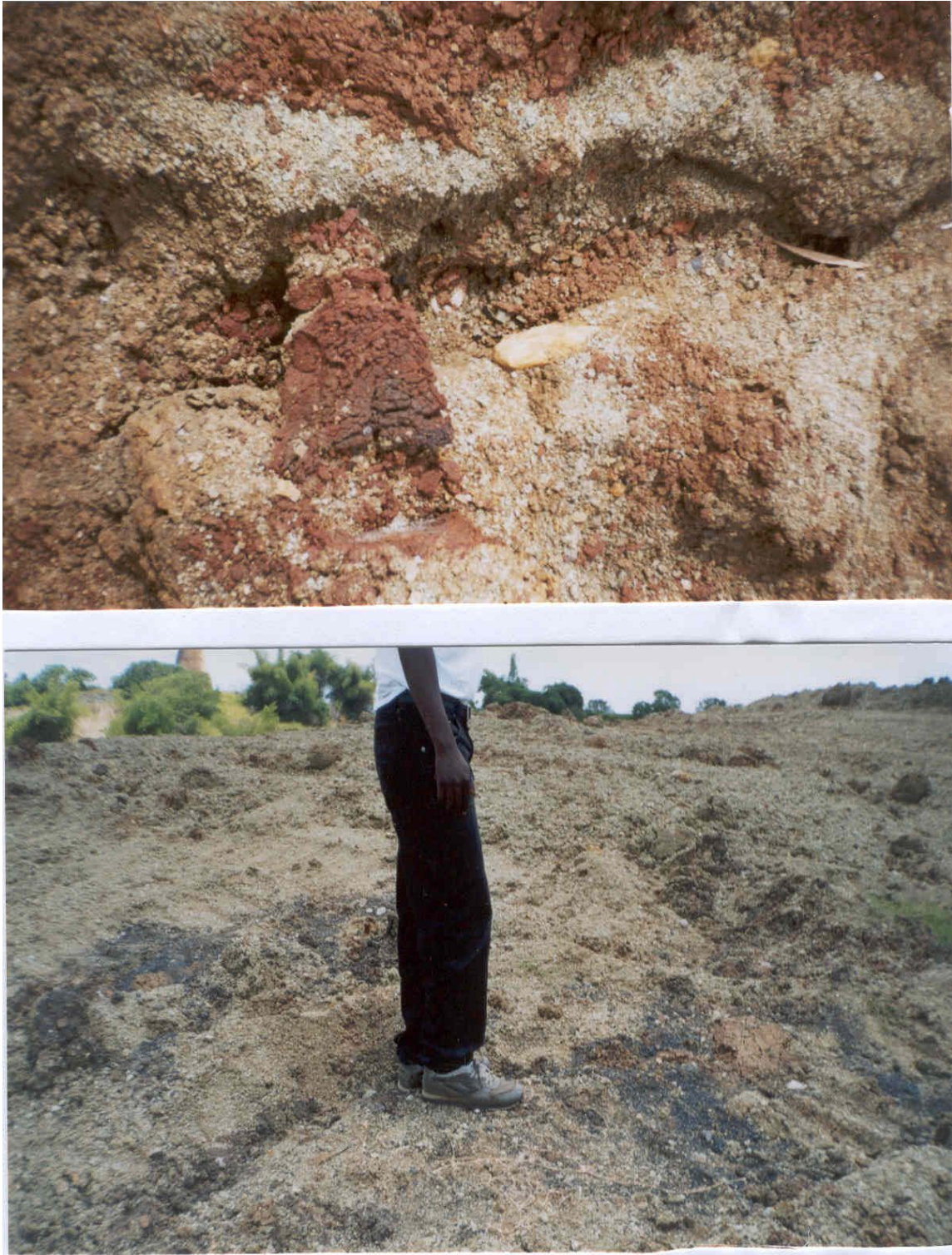
Photo 8.2 – Shows contaminated soil (reddish feature with slag residue) and Photo 8.3 (below) showing an erosion process rediscovering the slag in the dam.
