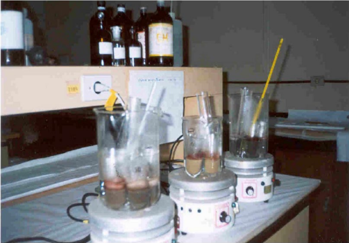
Photo 4.4 – Shakers with Beker containing the test tubes with the reducible phase solution.
