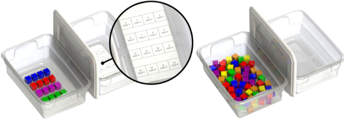
Figure 2.18: (Left) M-BBT and T-BBT-block templates following the test template. (Right) BBT-100 blocks randomly placed inside a bin (MORGAN et al., 2019).
