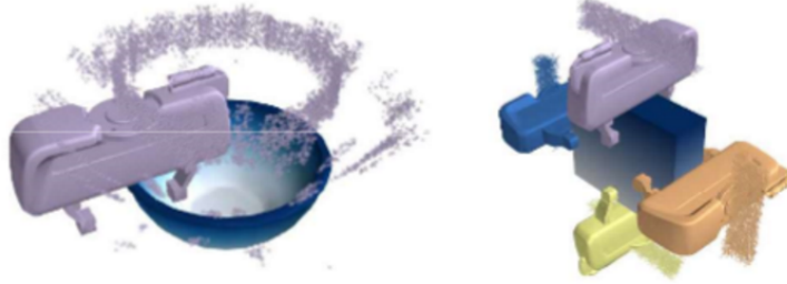
Figure 2.6: The grasp sampling simulation used by Mousavian, Eppner and Fox (2019) and Murali et al. (2020). The FleX sim (VICENT et al., 2016) was used to sample the grasps.
