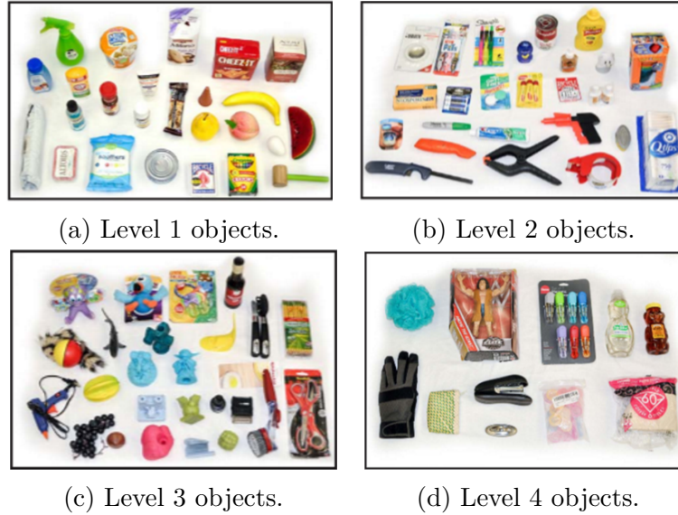
Figure 2.14: (a) Level 1 objects consisting of prismatic and circular solids (b) Level 2 objects including clear plastic and household objects with a lower level of graspability. (c) Level 3 objects with adversarial geometry and material properties (d) Level 4 objects with different reflectances and material properties which affect the ability to form a vacuum seal on the object surface (MAHLER et al., 2019).
