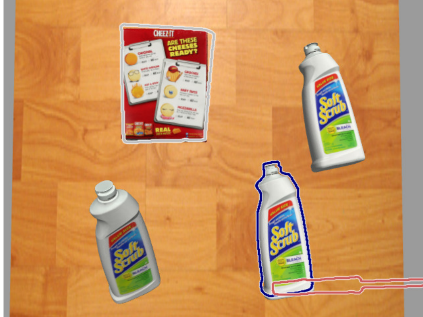
Figure 2.7: Single instance object detection and pose estimation with false positive object detection.
