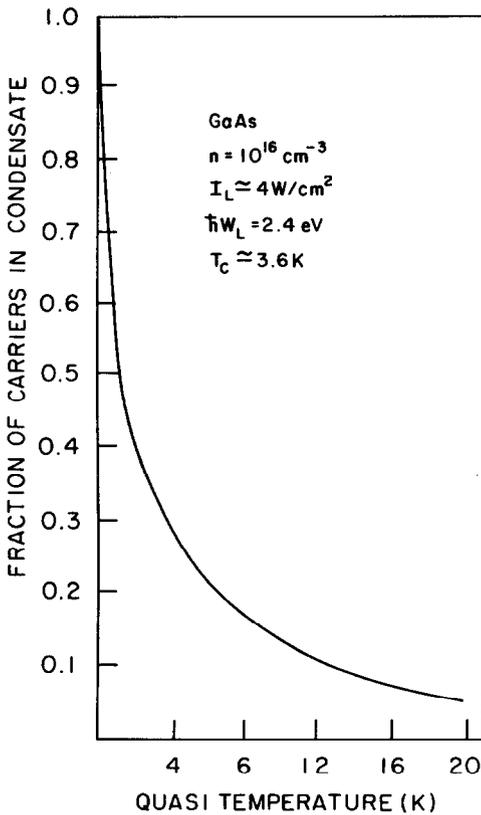
Fig. 2: Fraction of carriers in the nonmetallic polarizable state as a function of carrier quasitemperature.
