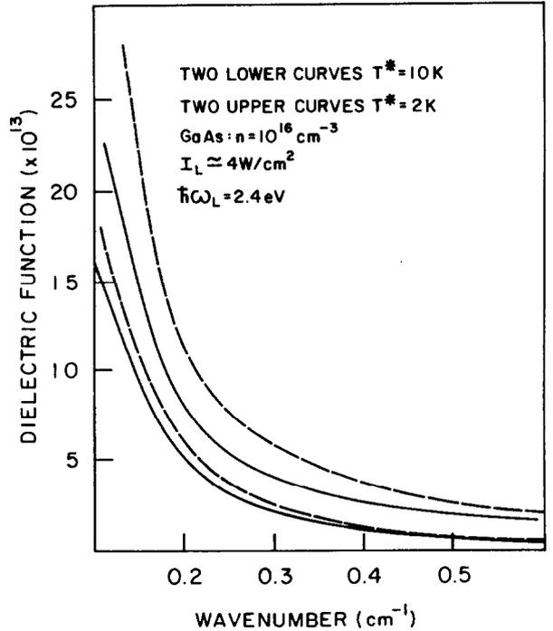
Fig. 1: The dielectric function of Eq. (6) (full lines) and Lindhart's dielectric function for the two component free carrier system (dashed lines).
